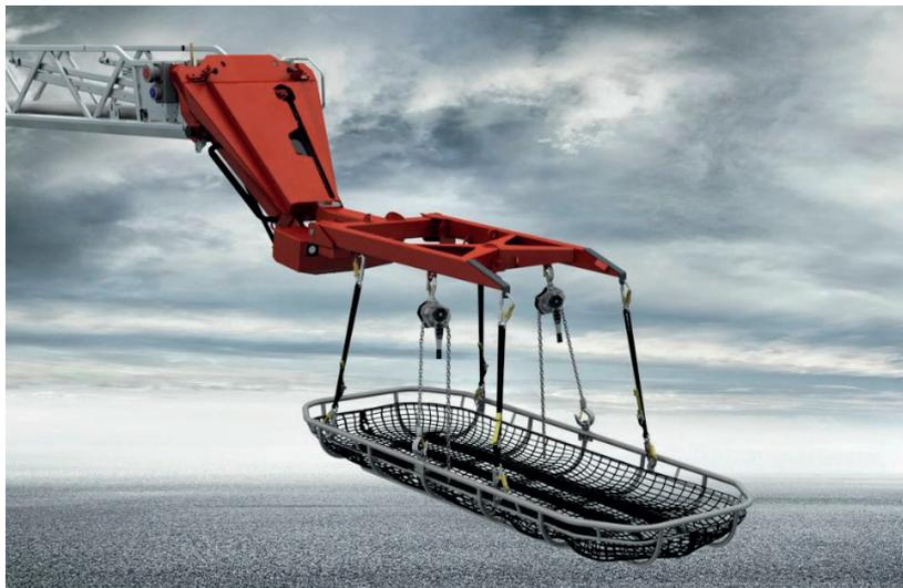
In the case of operation, the arm enters the space in which the patient is located via a suitable opening. The movable support frame allows at any time - even if the ladder truck is not parked parallel to the house - for a perpendicular retraction or extension relative to the house wall. The leveling of the support arm is automatic, depending on the angle of elevation of the ladder. These features provide a maximum of safety and comfort for both, patient and firefighter.
