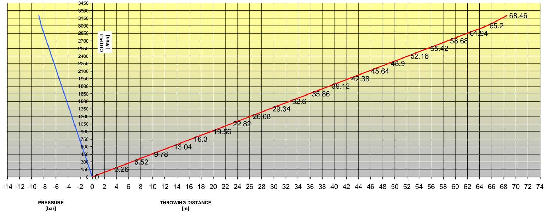
Monitor performances with: Wind +/- 0 m/sec; Monitor elevation angle + 30/35°; Pump suction from tank; Water temperature +15°C; Barometric pressure 1013,25 hPa
