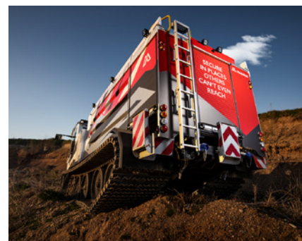
High payload, minimum ground pressure: 30 times less pressure than a 6x6 truck
