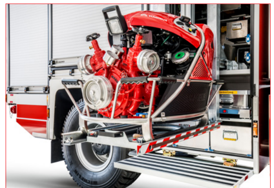
Portable pump storage
