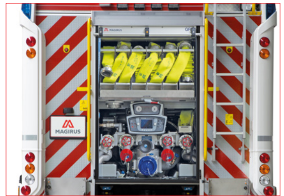
360 m B-hoses layer fitting at the vehicle rear
