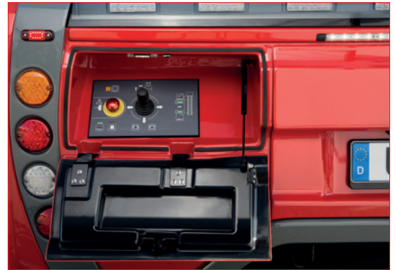
Supporting control panel with cover
