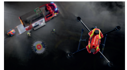
Tracking mode: Camera with AI identification and tracking of up to 10 objects (vehicles and people)
