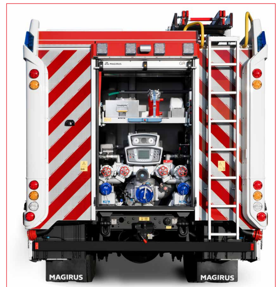
Readily accessible pump with intuitive HMI panel
